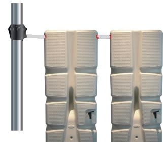
It is enough to place one second tank on the first. You need for this: 1 pipe Ø 20mm interior + 2 connector tips. Bore the filling hole opposite to the one connected to the collector and bore also the filling hole on the second tank. Put the connecting tips on the both tanks and connect them with the pipe.
