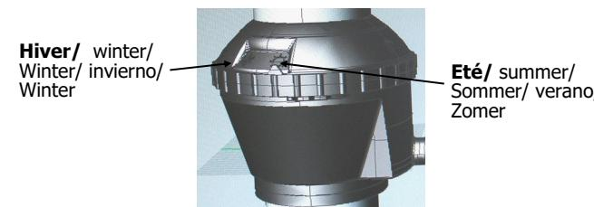
Care, the filling system of the tank works only if the kit placed on the rain pipe, is in position "opened". Position called "summer", symbolized by the "sun". Conversely, in order to stop the filling, put the kit on position "closed", symbolized by the "ice crystal".
